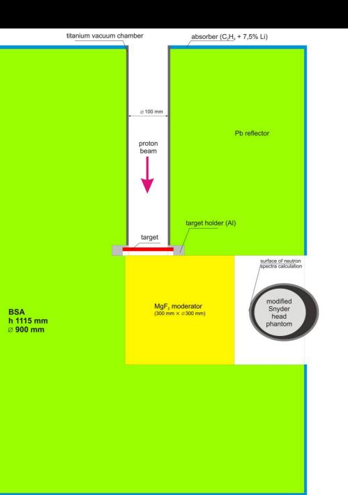
Orthogonal mode @ 2.5 MeV Dose rate @ 10 mA = 3 RBE Gy / min AD = 12 cm TR = 4 advantage: 1. high dose rate
