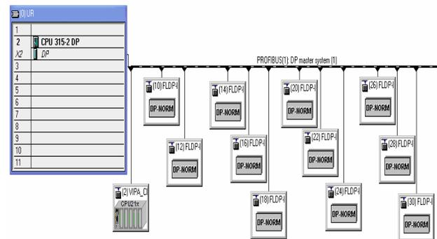
Figure 2. PLC controller with Profibus protocol.
