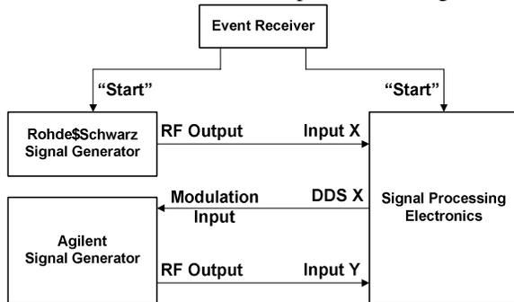
Fig.5. Scheme of Lab test of TMS electronics.
