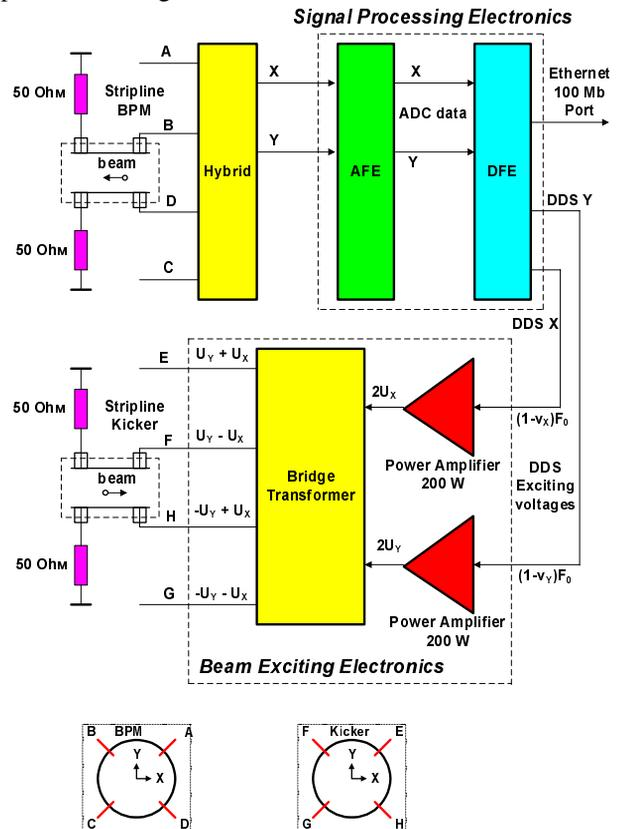
Fig.1. The structure of the Tune measurement system.
