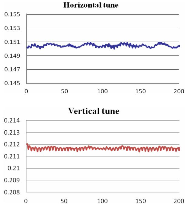
Fig.6. Results of horizontal (upper) and vertical (lower) tune measurements with beam at VEPP-3 at  $\sim 1.8$  GeV.
