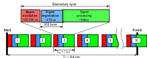
Fig. 4. Time diagram of the whole measurement cycle.
