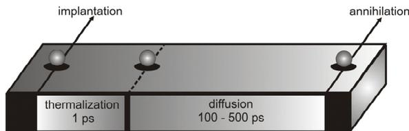
Figure 1: Stages of positron implantation into the matter.
