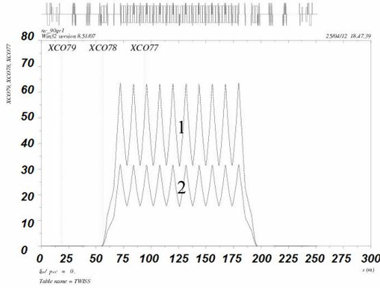
Figure 1: Closed orbits of ion beams 1 — Au<sup>77+</sup> and 2 — Au<sup>78+</sup>; the closed orbit of Au<sup>79+</sup> bare nuclei coincides here with abscissa axis.
