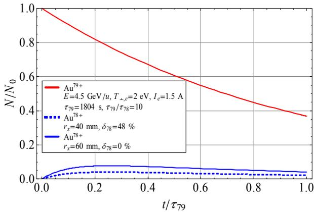
Figure 5: Solution (6) for beam energy  $E = 4.5$  GeV/u.
