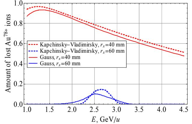
Figure 2: Loss factor  $\delta_{78}$  of ion beam Au<sup>78+</sup> as function of beam energy  $E$ .
