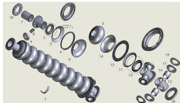
Figure 4: Mechanical design of e-LINAC nine-cell cavity
