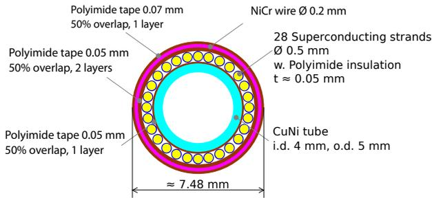
Figure 2: The cable of the corrector magnets.
