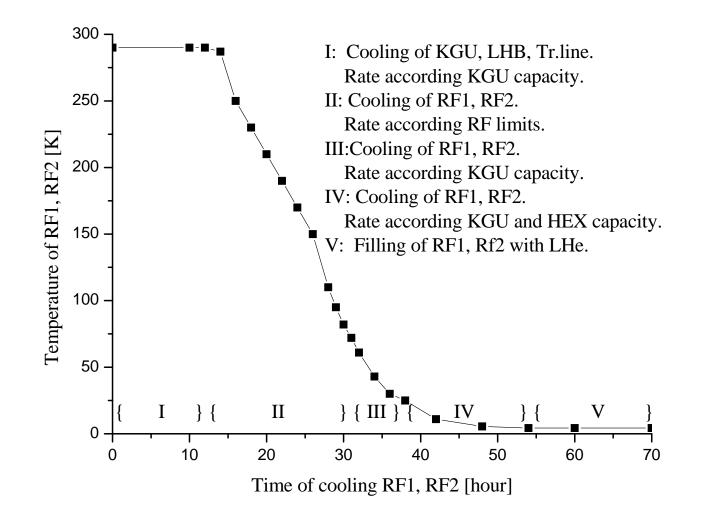
Cooling down of the RF separator superconducting cavities by CVS.
