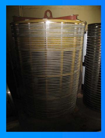
Maximal voltage – 900 V Maximal current – 900 A Inductance – 0.24 mH 16 turns with water cooling Frequency – 640 Hz
