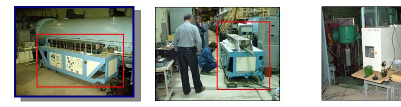
IHEP laser (CO<sub>2</sub>, 2.7 J, 10  $\mu$ m, 0.25 Hz)
