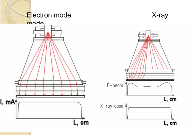
Due to the special magnetic lens the beam profile may be formed along the output window.
