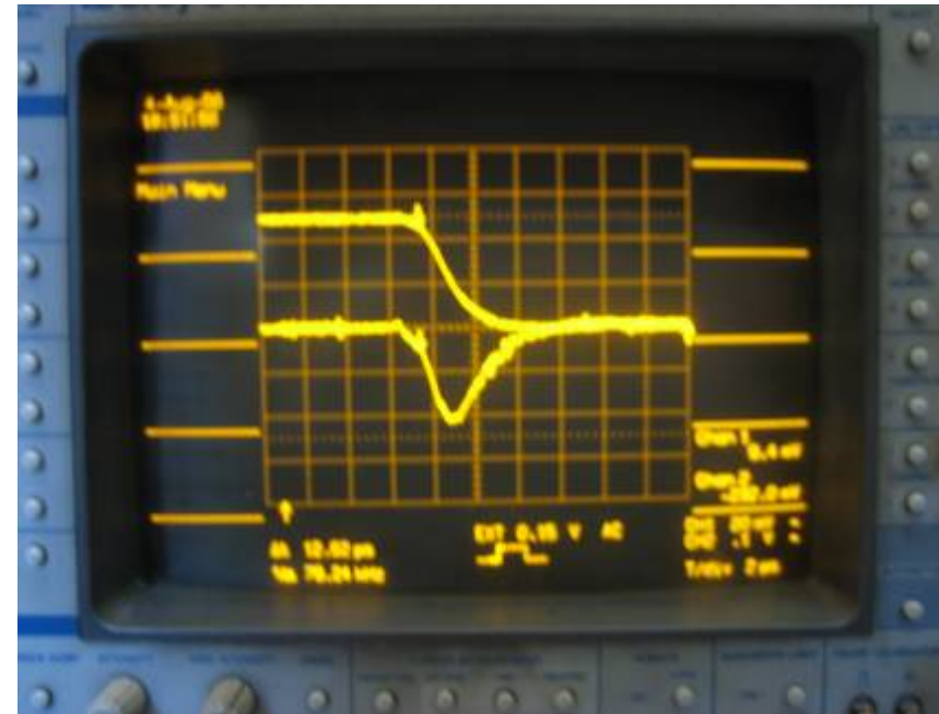
Stored electrons extracted to the collector
