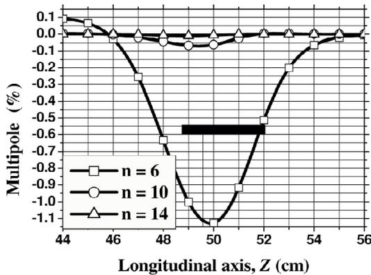
Figure 3: Multipoles  $b_6$ ,  $b_{10}$ ,  $b_{14}$  along longitudinal axis.
