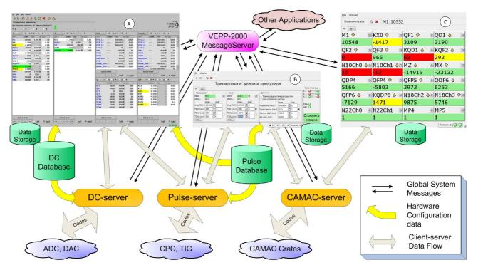
Figure 5: VEPP-2000 injection channels automation system layout. Three servers and three GUI applications provide needed functionality for channels tuning. "Global System Messages" allows to the application to exchange with messages about mode changing, different global settings changing, failures, etc.
