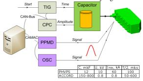
Figure 2. Schematic and main parameters of pulsed power sources. PPMD - pulsed parameters measurement device - integrating ADC.
