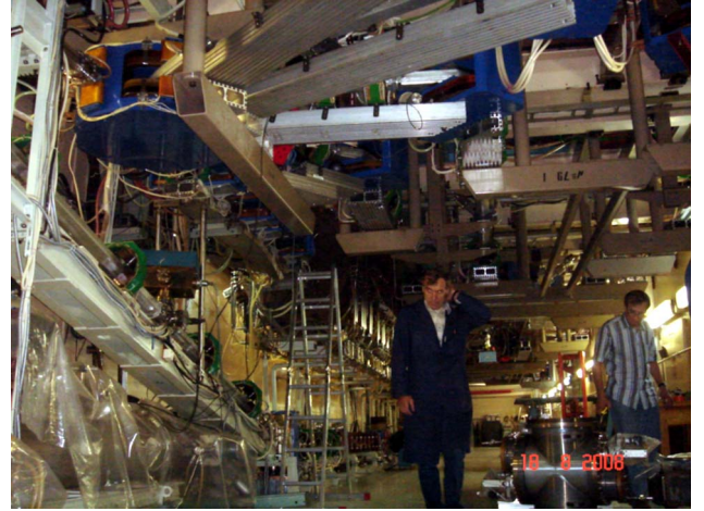
Figure 6: The bends are hanged on the ceiling. Round magnet is at the top left corner, the old terahertz FEL magnetic system is at down-left. Elements of the optical resonator for the second-turn FEL are yet at the floor (down-right corner).
