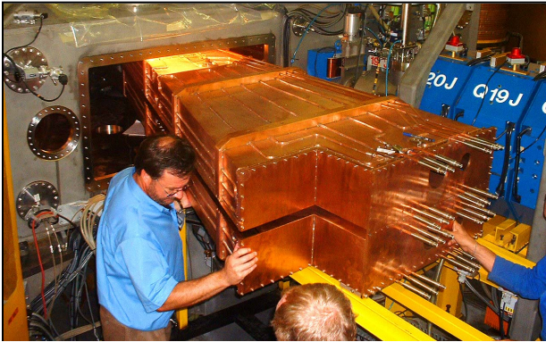
Figure 5: The flat-topping resonator of the SSC.
