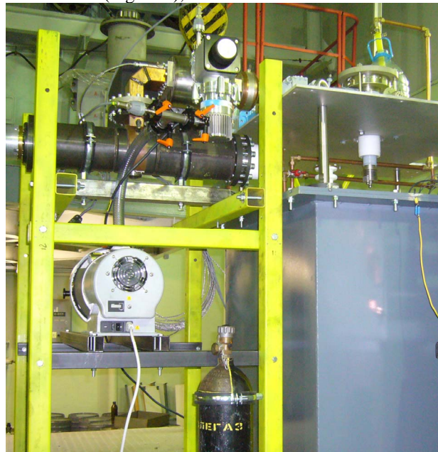
Figure 4: Linac assembly and the modulator.
