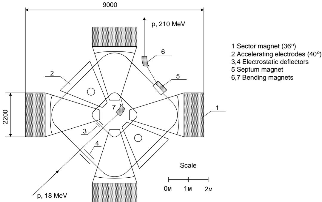
Figure 1: The RC-18/210 ring cyclotron
