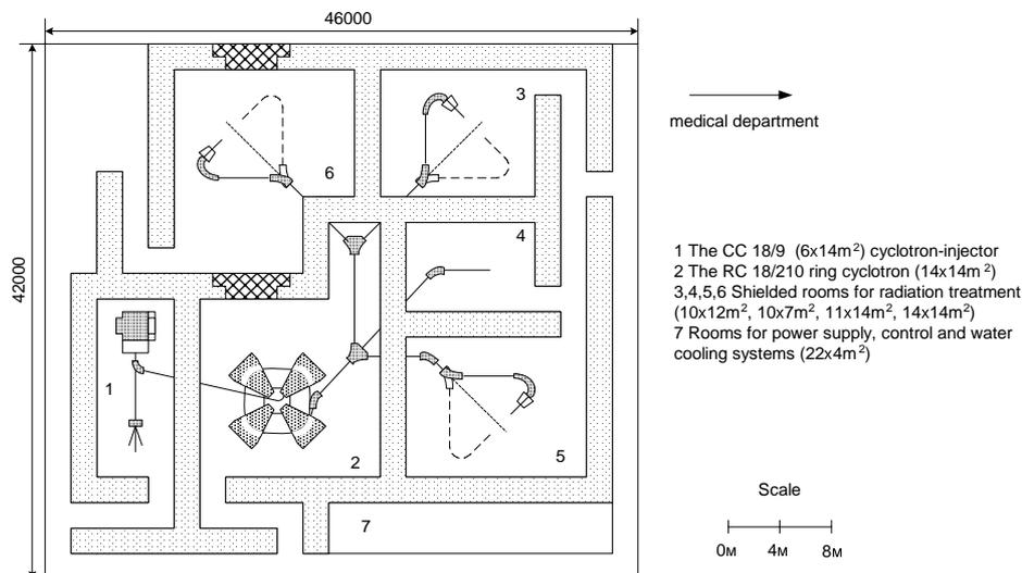
Figure 2: The system for proton therapy. Layout of the equipment.
