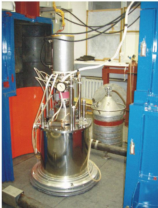
Fig. 3. Photo of the upper part of the stand. Visible components: cryomagnet, calorimeter, part of the biologic protection.
