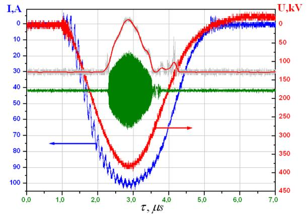
Fig. 5. Oscillograms of the current, voltage, and power envelope of the output microwave radiation, and of the corresponding signal from the mixer (green line). Signal parameters are  $U = 395$  kV,  $I = 100$  A,  $P_{out} = 10$  MW, and efficiency = 25%.
