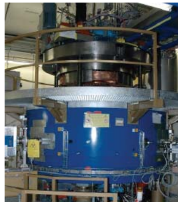
Fig.6 PSI new superconducting proton medical cyclotron constructed by Accel.
