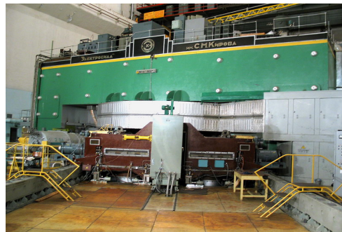
Fig. 1 JINR synchrocyclotron applied for proton therapy.
