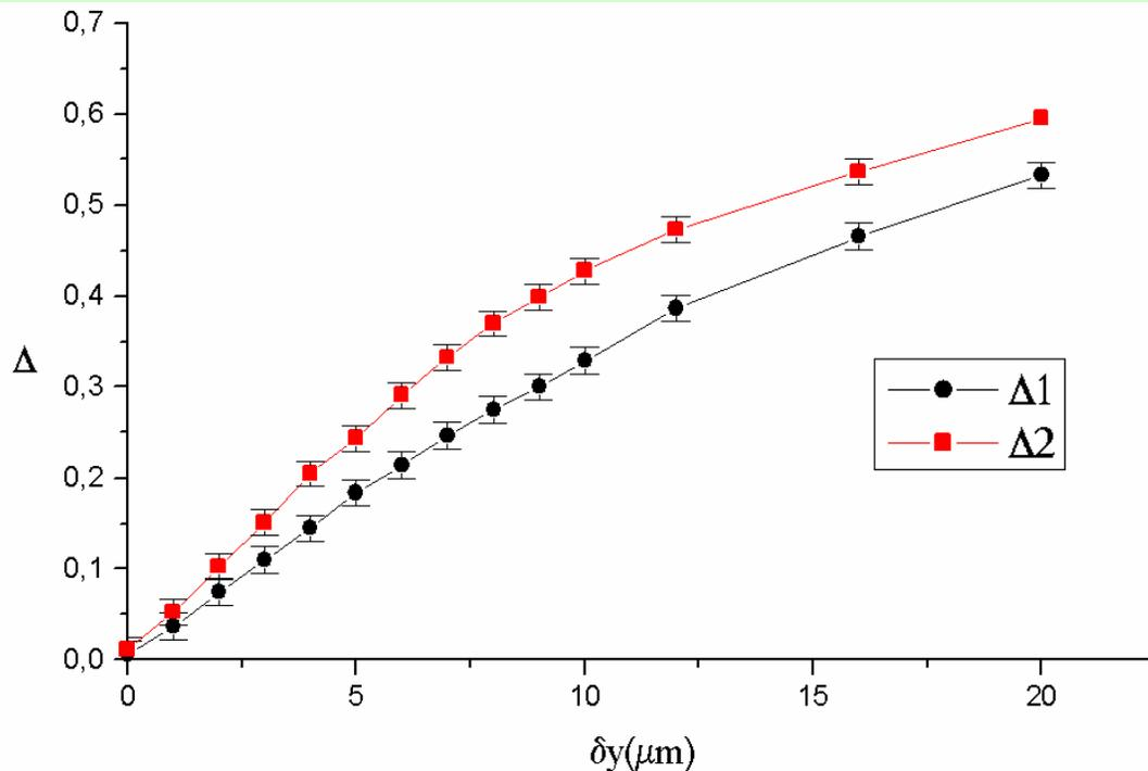
The image asymmetry dependence on the bunch tilting amplitude
