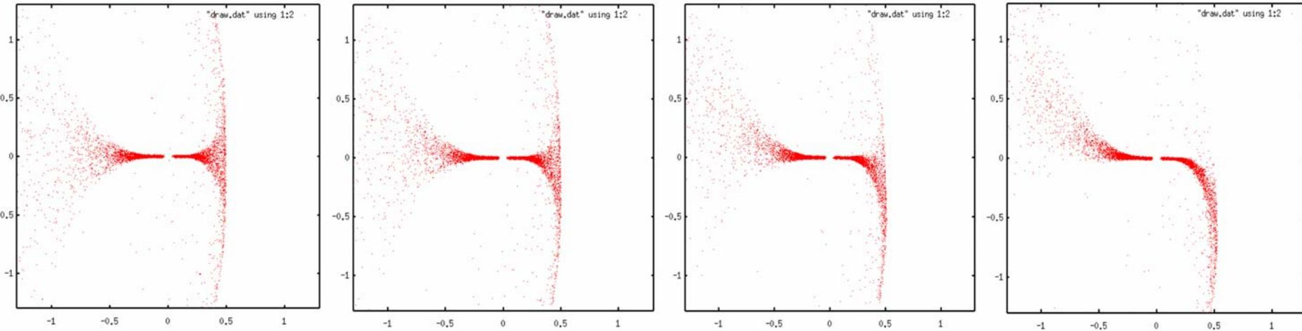
**Screen images for increasing amplitude of the bunch tilt  $\delta y$ .**
