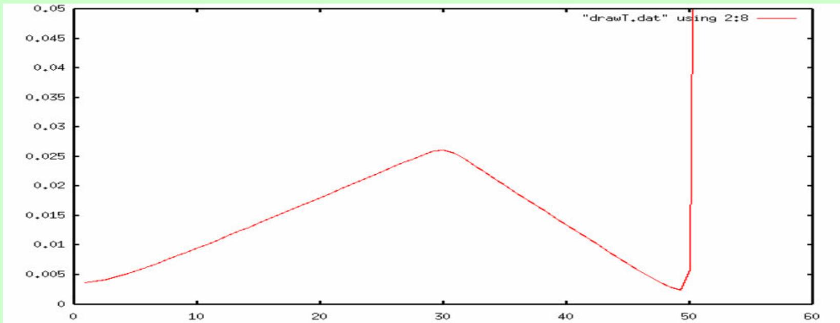
The probe beam envelope from the gun exit to the screen (horizontal axis (cm)), interaction point is placed 2 cm before the screen. The vertical axis gives the RMS transverse probe beam size in cm (probe beam is round).
