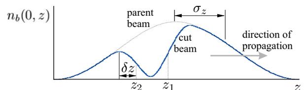
Figure 1: Beam shape at the entrance to the plasma.
