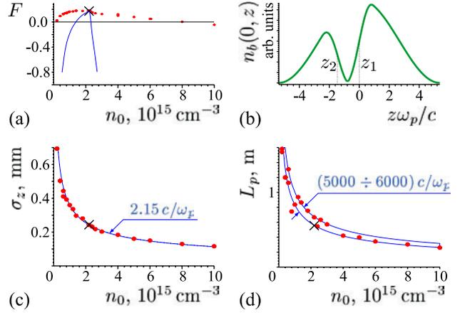
Figure 2: (a) Values of the criterion function on the optimum curve (dots) and on the line  $(\sigma_r, \sigma_z, z_1, z_2, L_p) = \text{const}$  (line); (b) optimum beam shape; (c) optimum beam length; and (d) optimum plasma length. Dots show the local maxima obtained numerically.
