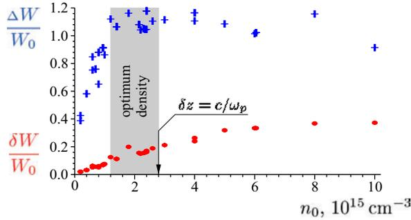
Figure 4: Dependence of the witness energy gain  $\Delta W$  (crosses) and energy spread  $\delta W$  (ovals) on the plasma density.
