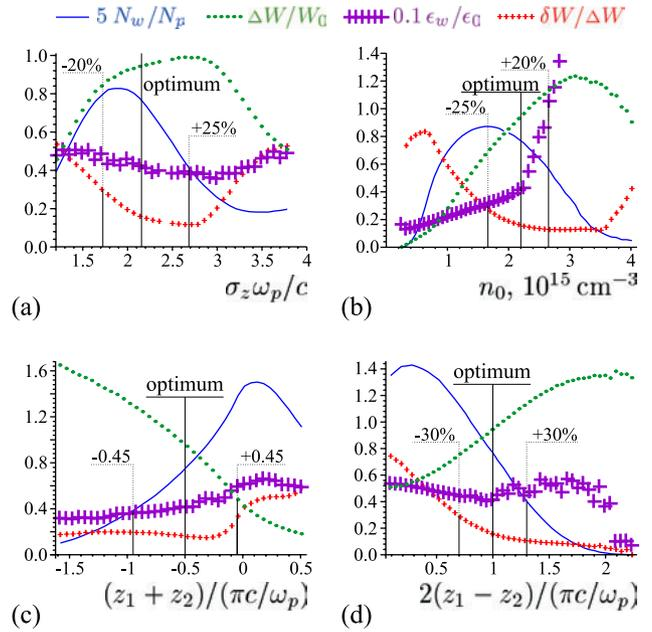
Figure 6: Variation of the witness population  $N_w$ , energy gain  $\Delta W$ , emittance  $\epsilon_w$ , and energy spread  $\delta W$  as (a) the parent beam length, (b) plasma density, (c) cut-out location, and (d) cut-out width deviate from the optimum values.
