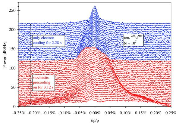
Figure 1: Longitudinal Schottky noise signal of combined stochastic and electron cooling of  $10^7$   $U^{92+}$  ions injected at an energy of 400 MeV/u. The stochastic pre-cooling is switched of after 3.1 s and electron cooling cools to minimum momentum spread.
