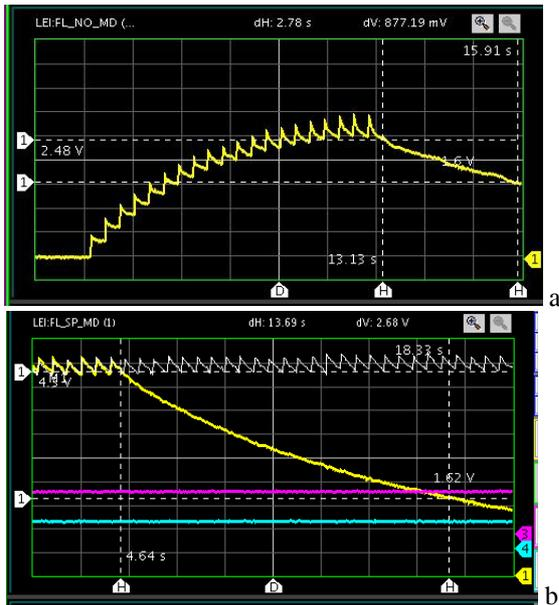
Figure 2: a- the ion beam accumulation for maximum density at center, b- the minimum density at center. The lifetime after stop of injection was 6.3 s for “a”. For “b” life time is 13.8 s.
