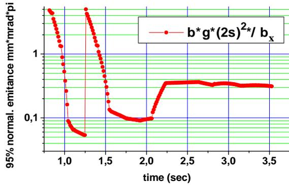
Figure 5: The normalized emittance (95%) variation versus time inside the magnet cycle.
