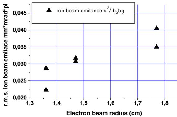
Figure 6: The equilibrium r.m.s. emittance versus the electron beam radius at drift section. The electron beam 0.1 A,  $U_{\text{contr}}=200$  V  $U_{\text{anode}}=900$  V.
