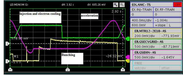
Figure 3: The standard magnet cycle of acceleration of ion beam: magento line is the magnet field value, green line is the anode voltage for the control of the electron beam current, yellow line is the number of ions at beam.
