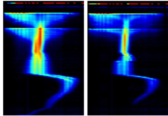
Figure 7: Comparison of cooling with different electron beam radii 1.78 cm and 1.37 cm. The cooling for the second injection is faster when the cooled ion beam from first injection presents.
