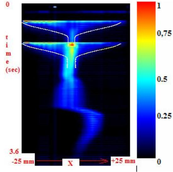
Figure 4: The change of the ion beam profile in LEIR cycle. Its initial moment shows the 2 injections and cooling, then acceleration from 5 MeV/u to 71 MeV/u. White colour lines show simulation made with “trubs.exe” code with the initial ion amplitude 25 mm.
