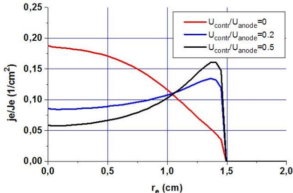
Figure 1: The profile of electron beam for different setting of the electrode voltage.
