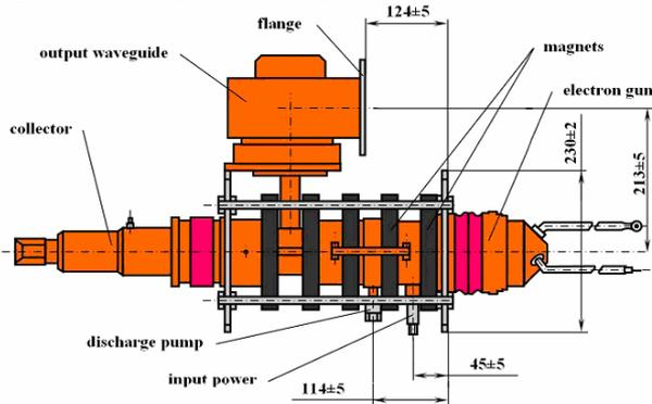
Figure 7: 1498MHz 15kW CW MB klystron with PPMFS.
