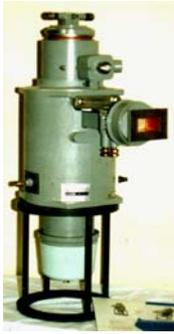
Figure 1: Pulsed MB klystron KIU-168
