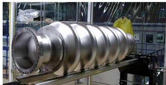
Figure 4: The ERL cavity following BCP at JLab.
