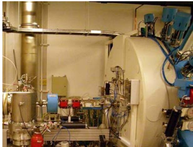
Figure 1: The CC-18/9 cyclotron with the external injection system.
