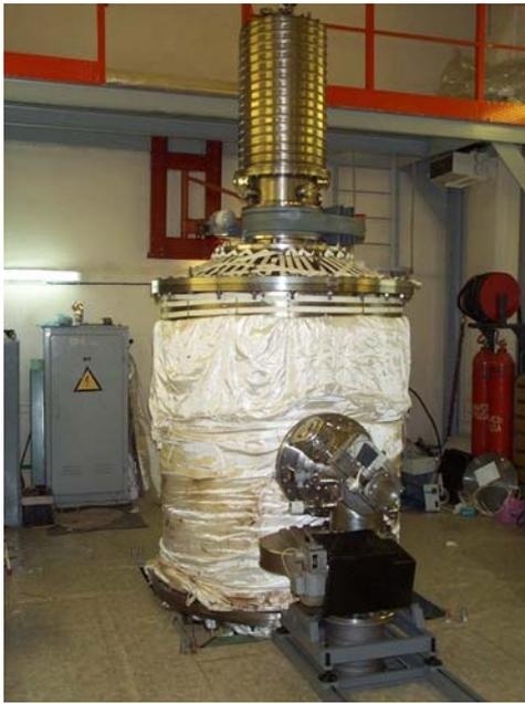
Figure 7: Vacuum tank and cryogenic pump.
