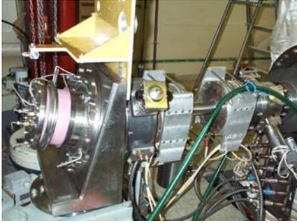
Figure 2: The H ion source and low energy beam tract.
