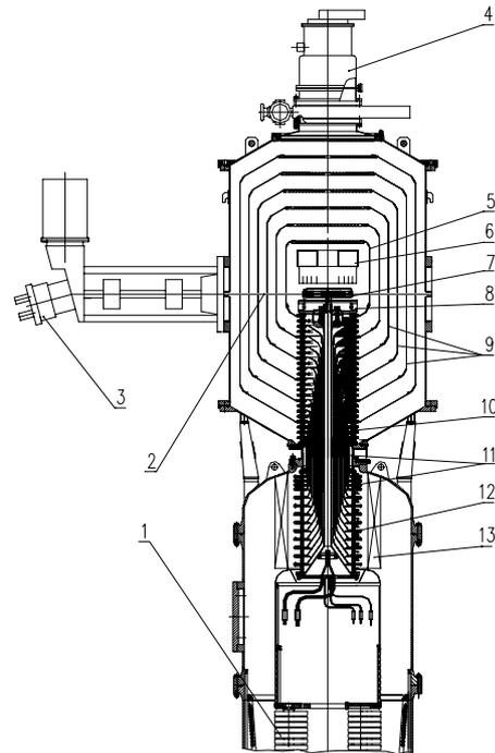
Figure 1: Vacuum insulation tandem accelerator.
