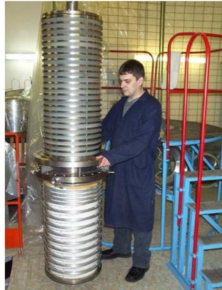
Figure 6: The high-voltage feedthrough.
