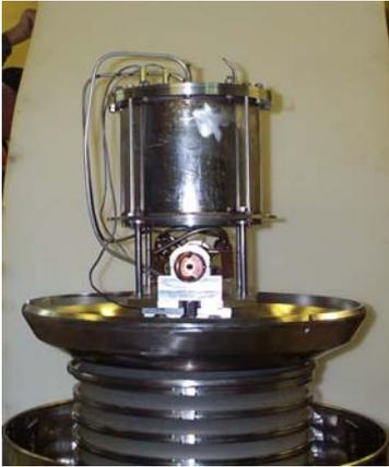
Figure 3: The pipe of charge-exchange target and volume of target's control systems.
