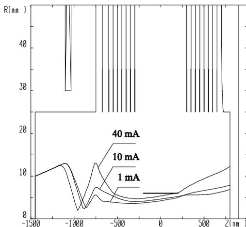
Figure 8: Example of computer simulation envelope results for some  $H^-$  beams.
