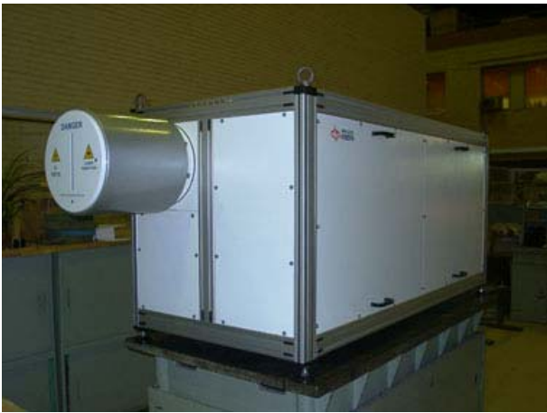
Figure 3: The primary collimator and the radiation source.
