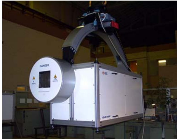
Figure 1: The irradiator of the UEL-15-D accelerator for radiography.
