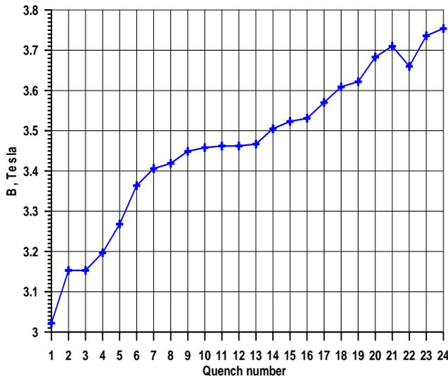
Figure 1: Quench history during bath wiggler test.
