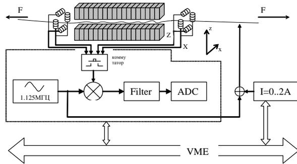
Figure 6: The scheme of the stretched wire method.
