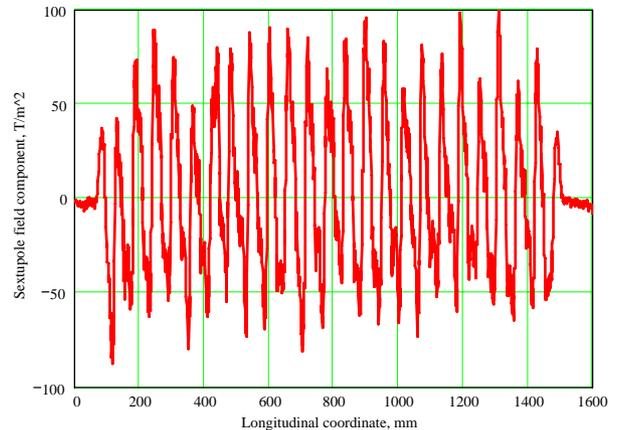
Figure 3: Field sextupole component along the wiggler estimated with use of 5 Hall probe array.
