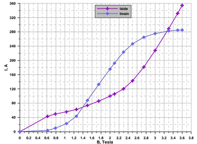
Figure 7: The currents  $I_{side}$  and  $I_{main}$  for zero first field integral versus magnetic field.
