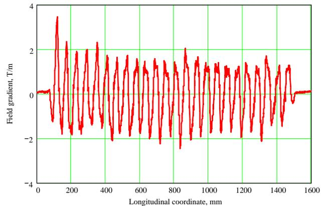
Figure 2: Field gradient along the wiggler estimated with use of 5 Hall probe array.
