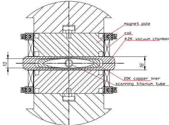
Figure 4: The copper liner and the tube position.
