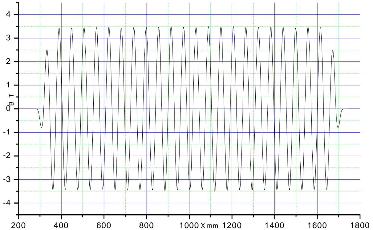
Figure 8: Longitudinal magnetic field distribution at 3.5 Tesla.
