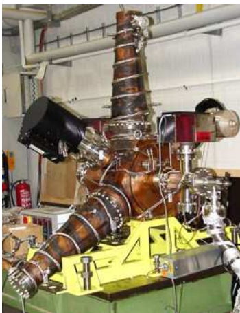
Figure 3: Prototype of the EU-HOM-Damped 500 MHz resonator ( R_s=3.1 \text{ M}\Omega , Q_0=27000 ).
