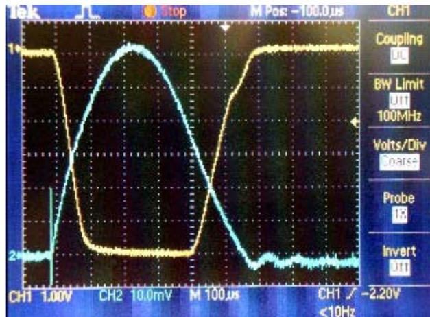
Figure 7: EVG output voltage and HV transformer input current 4kV/div; 2A/div.
