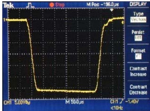
Figure 5: HV -400kV pulse.
