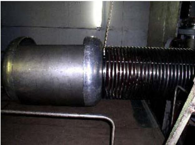
Figure 4: The accelerating tube with the IS high-voltage dome.
