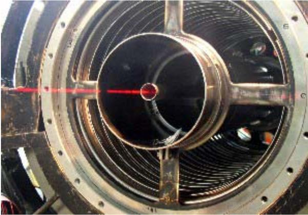
Figure 3: The accelerating tube EOS alignment.
