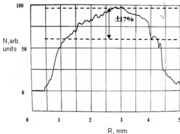
Figure 5: Radial electron density distribution of beam.
