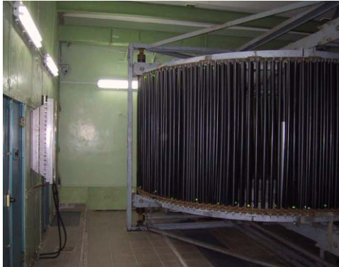
Figure 3: Irradiation zone for products.
