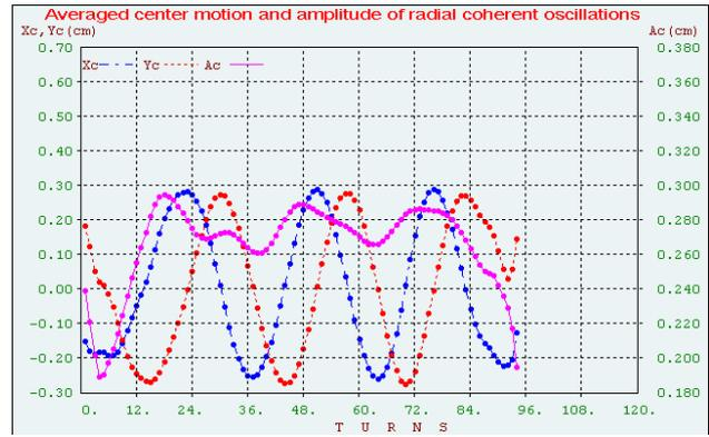
Figure 6: Radial oscillations and average center motion for measured field map without first harmonic.
