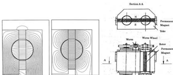
Figure 2: Principle of Flux Engine and its drawing.
