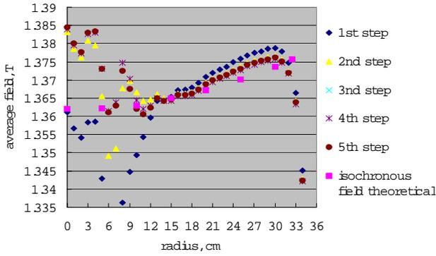
Figure 4: Series of average field measurements to reach isochronous field.
