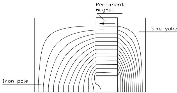
Figure 1: PM cyclotron magnet cross-section (1/4 part is shown)
