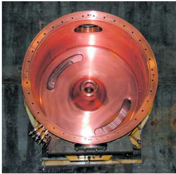
Figure 3: Accelerating structure assembled in the bunker.
