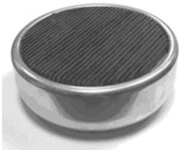
Figure 2: “Blade” metallodielectric cathode 100mm diameter.
