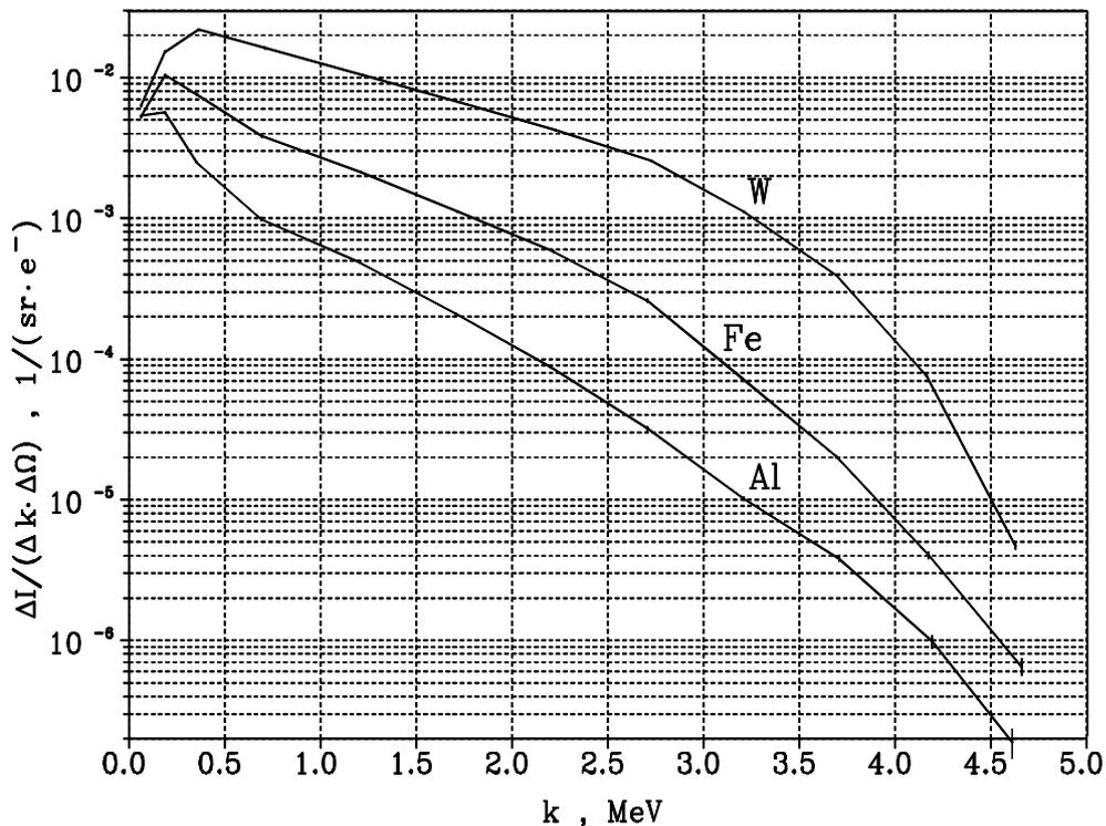
Figure 1: Energy distribution of photon radiation from aluminum, iron and tungsten targets to the angle escape interval  $123.75^\circ \dots 135.0^\circ$ ,  $E_0 = 5$  MeV.
