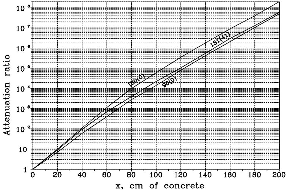
Figure 3: Attenuation by concrete of the air kerma of bremsstrahlung from the Al target,  $E_0 = 5$  MeV (see text).
