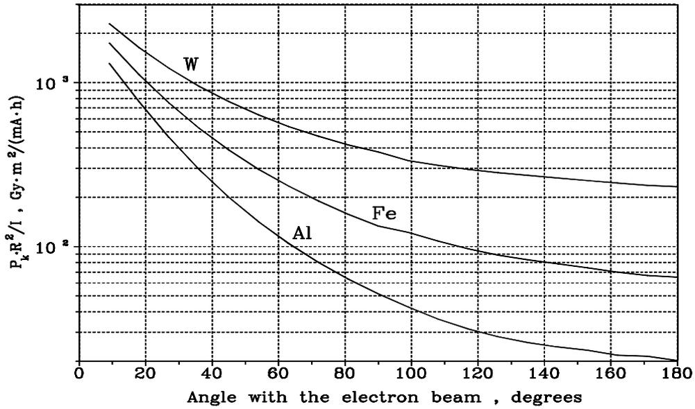
Figure 2: Angular dependences of the air kerma of bremsstrahlung from the targets,  $E_0 = 5$  MeV.
