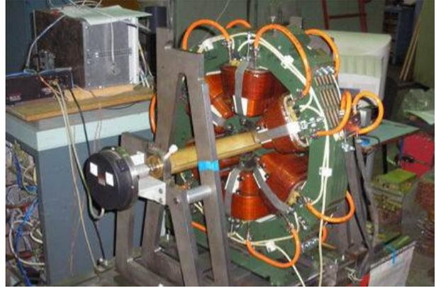
Figure 4: Rotating coil system with SRS magnet.
