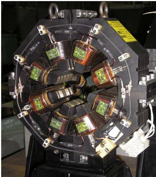
Figure 3: MLS SR octupole magnet.
