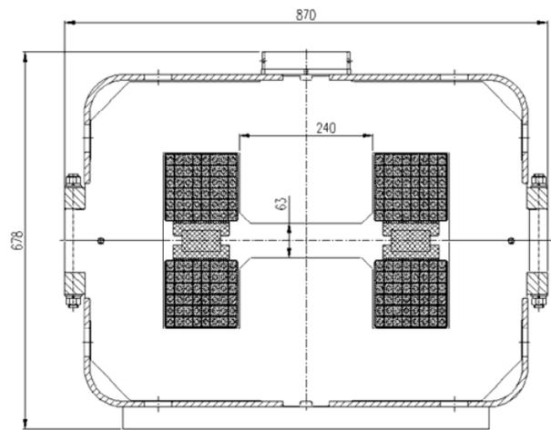
Figure 1: Cross-section of the MBXW magnet. The pole distance measures 63 mm. In order to achieve a good field region of  $\pm 41$  mm width with a high field
