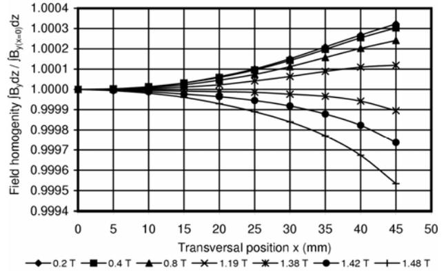
Figure 4: Field homogeneity of the integral magnetic flux density at different field levels after correction of the end chamfers (3D calculation, the groove is 3 mm × 40 mm).
