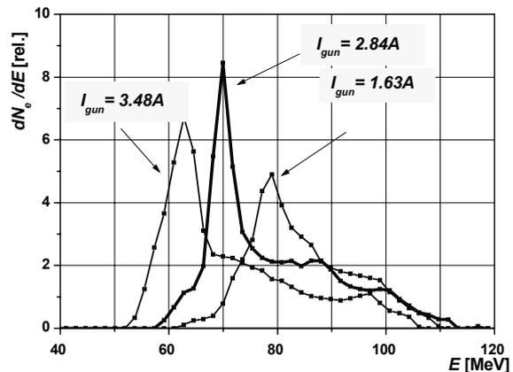
Figure 2: Energy spectra of the electron beam after acceleration in two sections for three values of gun beam current  $I_{\text{gun}}$ . The bold line shows the spectrum of the beam with maximum energy content.
