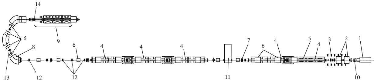
Figure 1: Lay-out of electron linac, isochronous turn and conversion system of injector complex VEPP-5. 1 — electron gun, 2 — subharmonic buncher, 3 — focusing coil, 4 — accelerating structure, 5 — solenoid, 6 — quadrupole lens, 7 — corrector, 8 — bending magnet, 9 — conversion system and first positron structure, 10 — wall current monitor, 11 — spectrometer, 12 — secondary-emission sensor, 13 — phosphor screen, 14 — Faraday cup.
