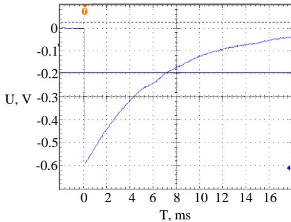
Figure 3: Faraday cup discharge signal. U – Faraday cup voltage, T - time.
