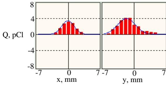
Figure 2: Beam profile monitor measurement results x and y - beam dimensions, Q – measured wire charge for histogram. curve – approximated Gaussian distribution.
