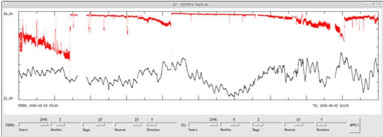
Figure 4: The out circuit cooling water temperatures during two and half months (red – out-stream temperature, black – in-stream temperature).
