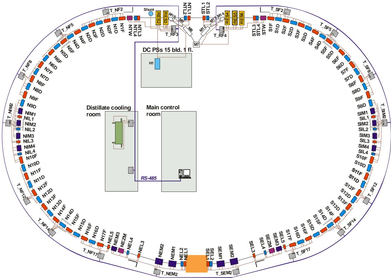
Figure 2: Scheme of the VEPP-4M temperature system.
