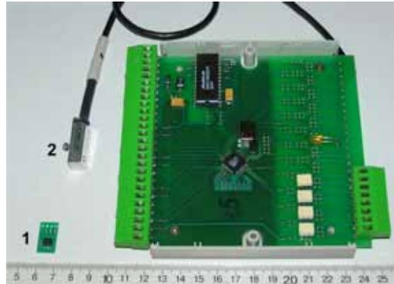
Figure 1: The temperature controller; 1 - sensor board; 2 – sensor inside the protection case.
