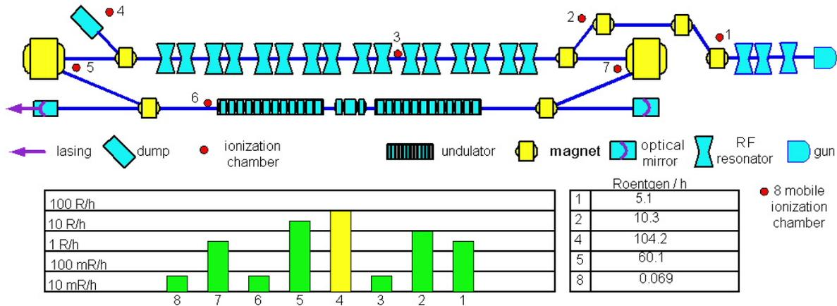
Figure 1: Arrangement of the radiation transducers in the accelerating hall.
