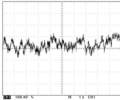
Figure 6: Amplifier noise (scale 100nV/div, 1sec/div).
