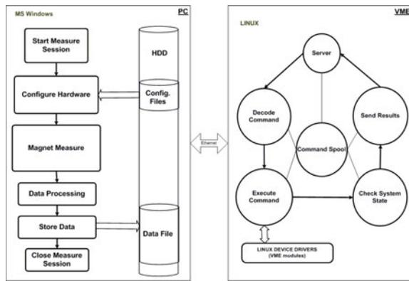
Figure 7: Software structure.
