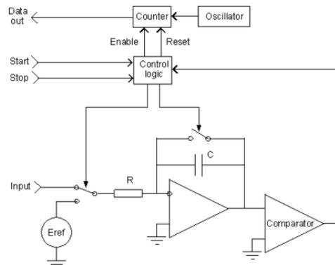
Figure 1: Simplified structure of VsDC.
