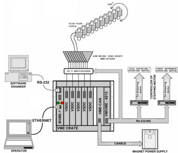
Figure 8: flip-flop coil measuring system structure.
