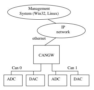
There are two alternative application schemes of the gateway. The first is remote CAN interface. The second is programmable logical controller (PLC).
