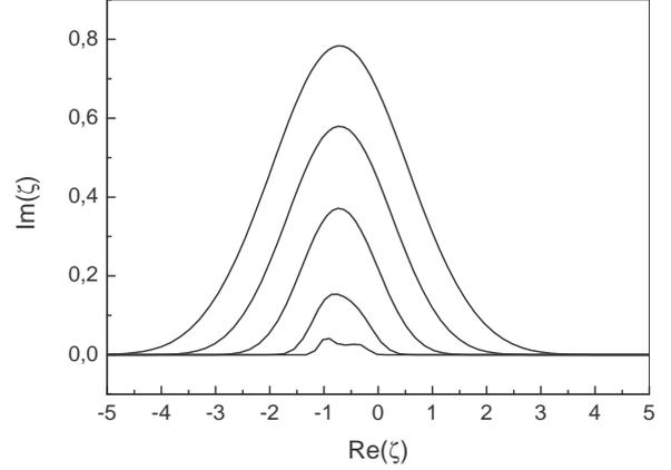
Figure 1: Stability diagrams for the vertical coherent oscillations ( $\zeta = \Omega_{m,n} / (\delta\omega_{ext})_{in}$ ). The oscillations are stable below the border curve,  $a = b = 0$ , from top to bottom  $(\sigma_p/\sigma_{in}) = 1, 0.75, 0.5, 0.25$  and  $0.1$ , no transverse cooling;  $m_x = 1$ .
