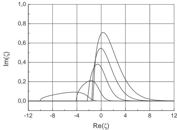
Figure 4: Stability diagrams for the vertical coherent oscillations. The oscillations are stable below the border curve,  $g = 0$ ,  $a = 0$ ,  $b < 0$ , flat beam ( $\epsilon_y \ll \epsilon_x$ ) from top to bottom ( $\epsilon_x/\epsilon_{in} = 1, 0.75, 0.5, 0.25$  and  $0.1$ ,  $q = 1$ ,  $m_x = 1$ ).
