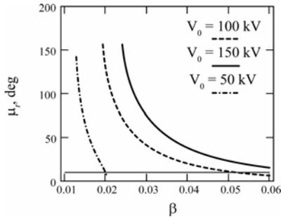
Figure 5: The phase advances  $\mu_r$  for different vane voltage  $V_0$ .
