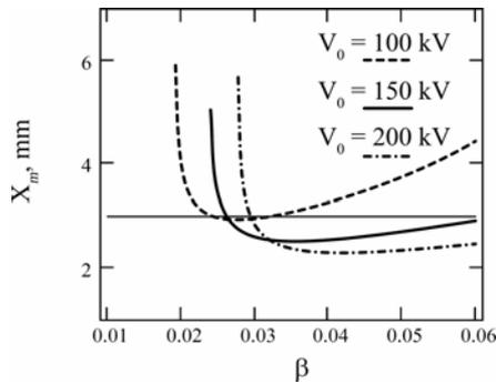
Figure 6: The beam envelop  $X_m$  as a function of the beam velocity  $\beta$  for different vane voltage  $V_0$ .
