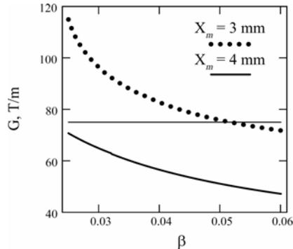
Figure 4: The magnetic field gradient  $G$  as a function of the beam velocity for two envelopes  $X_m$ .
