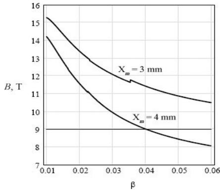
Figure 2: The focusing magnetic field  $B_{min}$  as a function of the beam velocity for two beam envelopes  $X_m$ .
