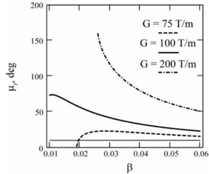
Figure 3: The phase advances  $\mu_r$  for different magnetic field gradient  $G$ .
