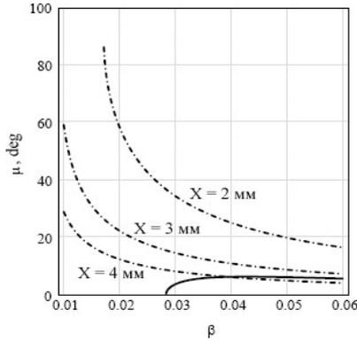
Figure 1: The phase advances  $\mu_r$  for different beam envelopes  $X_m$ .
