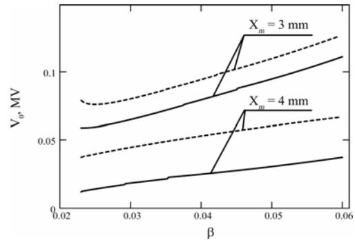
Figure 7: The voltage of the electric quadrupoles as a function of the beam velocity for two envelopes  $X_m$ . The solid lines correspond to case  $\phi_1 = -\phi_2 = -20^\circ$ ; the dash lines correspond to case  $\phi_1 = -30^\circ, \phi_2 = 20^\circ$ .
