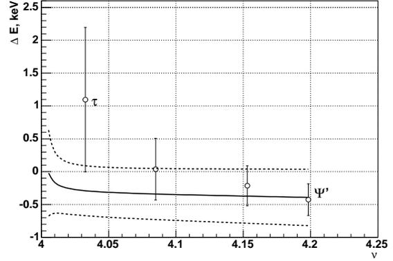
Figure 2: Energy shift versus spin tune at 1 mm vertical orbit RMS. Circles with errors are results of simulation, solid line presents the estimation by equation (12) and dashed line is the estimation uncertainty by (14).
