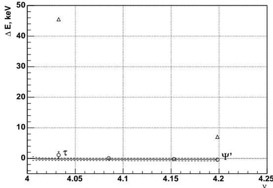
Figure 1: Energy shift versus spin tune at 1 mm vertical orbit RMS. Triangles are calculations neglecting correlation term, circles with errors are results of simulation, solid line presents the estimation by equation (12) and dashed line is the estimation uncertainty by (14).
