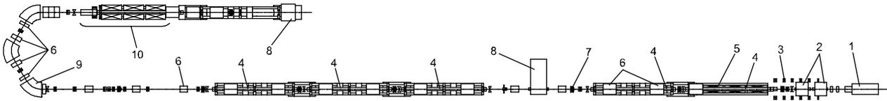
Figure 3: Part of injector complex is in operation now: 1 — electron gun, 2 — sub harmonic bunching system, 3 — focusing coil, 4 — accelerating structure, 5 — solenoid coil, 6 — quadrupole lens, 7 — corrector, 8 — spectrometer, 9 — bending magnet, 10 — positron production system and first accelerating structure of positron linac.
