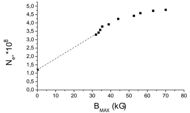
Figure 5: The dependence of positrons number upon the maximum field in matching device. Driving electron beam energy — 265 MeV, number of electrons in the primary electron beam —  $1.8 \cdot 10^{10}$ .
