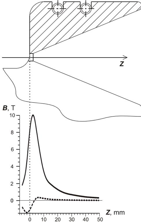
Figure 4: Results of magnetic measurements for matching device of VEPP-5 Injection Complex: upper curve — longitudinal magnetic field on the geometrical axis of the device, lower curve — transverse component of magnetic field on the geometrical axis Z.
